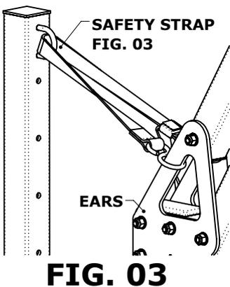
**STEP 03: TURN THE WINCH HANDLE CLOCKWISE TO RAISE THE LIFT UP AND OUT OF THE ANCHOR. IF THE LIFT WON'T MOVE, SHAKE THE MAST OF THE LIFT TO LOOSEN IT IN THE ANCHOR AND TURN THE HANDLE UNTIL THE LIFT COMES OUT OF THE ANCHOR. RAISE THE LIFT UNTIL THE STEM IS AN INCH OR TWO ABOVE THE FLOOR. THE LIFT IS READY FOR TRANSPORTATION. (FIG. 04)**
