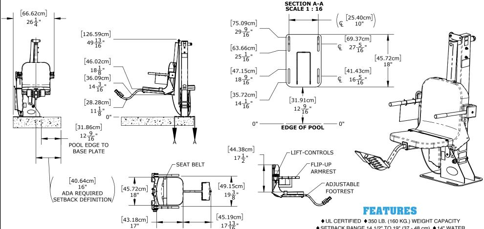
♦ SETBACK RANGE 14 1/2" TO 19" (37 - 48 cm) ♦ 14" WATER DRAFT ♦ FIELD REVERSIBLE ♦ ADJUSTABLE BASE PLATE ♦ FLIP UP ARMREST ♦ ALL STAINLESS STEEL CONSTRUCTION ♦ DURABLE POWDER COAT FINISH ♦ RECHARGEABLE BATTERY & WALL MOUNT CHARGER ♦ FIVE YEAR STRUCTURAL WARRANTY ♦ FIVE YEAR PRO-RATED ELECTRONICS WARRANTY
