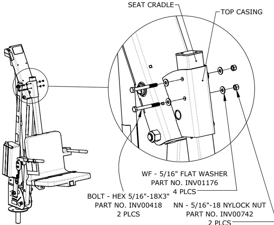
STEP 2) SLIDE THE SEAT CRADLE ASSEMBLY UP THROUGH THE TOP CASING OF THE MAST ASSEMBLY AND CONNECT USING THE SUPPLIED 5/16" HEX BOLTS, WASHERS AND NYLOCK NUTS. FOR STANDARD POOL CONFIGURATION THE SEAT CRADLE WILL BE CONNECTED AT THE TOP TWO HOLES. HOWEVER, THE SEAT CRADLE CAN BE ADJUSTED UP TO 6" HIGHER, IN 2" INCREMENTS, IF THERE IS A NEED FOR IT.
