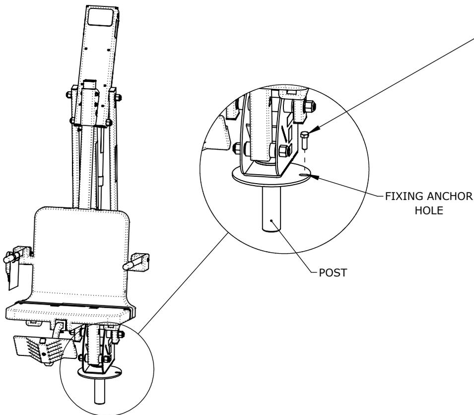
STEP 1) LIFT THE MIGHTY 600 MAST ASSEMBLY FROM THE SHIPPING CONTAINER. INSERT THE 1.90" [48mm] POST OF THE MAST ASSEMBLY INTO THE DECK ANCHOR. EASE THE MAST ASSEMBLY DOWN UNTIL IT RESTS ON THE DECK SURFACE. ROTATE THE BASE UNTIL THE FIXING ANCHOR HOLE LINES UP WITH THE FIXING ANCHOR. INSTALL THE 1/2"-13X1 1/2" HEX BOLT AND WASHER (PROVIDED IN THE STOCK BOX) TO HOLD DOWN THE LIFT. TIGHTEN THE BOLT.
