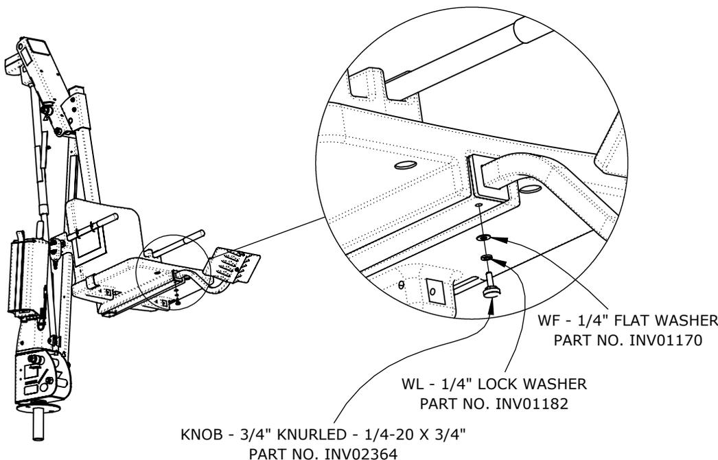
STEP 3) INSERT THE FOOTREST ASSEMBLY INTO THE 2"X2" SQUARE TUBING THAT SUPPORTS THE SEAT UNTIL THE PLASTIC INSERT OF THE FOOTREST ASSEMBLY SITS FLUSH AGAINST THE END OF THE 2"X2" TUBE. USING THE SUPPLIED 1/4" HARDWARE, FASTEN THE LEGREST ASSEMBLY TO THE 2"X2" TUBING.
