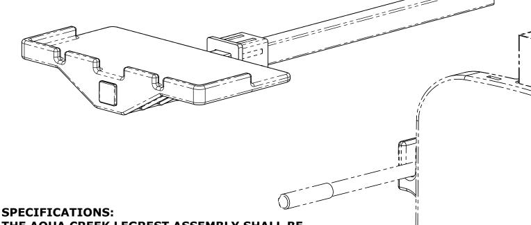
THE AQUA CREEK LEGREST ASSEMBLY SHALL BE **EXTENDABLE TO ACCOMMODATE A WIDE RANGE OF** USERS. THE LEGREST TUBE SHALL BE CONSTRUCTED OF TYPE 304 STAINLESS STEEL. THE FOOTREST SHALL BE MOLDED FROM HDPE WITH A UV ADDITIVE. THE FOOTREST IS ALSO AVAILABLE IN TAN, WHITE AND **GRAY.**
