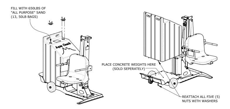
\*NOTE: DO NOT OVER TIGHTEN BOLTS. OVER-TIGHTENING CAN CAUSE DAMAGE AND COMPROMISE THE SAFETY OF YOUR LIFT.
