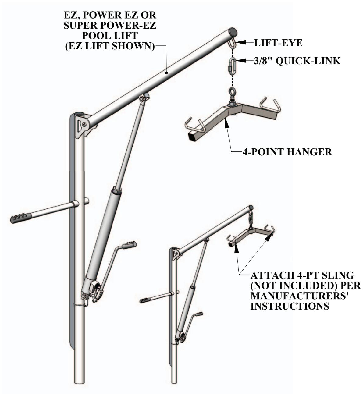
The 4-POINT HANGER BAR comes fully assembled, and only needs to be attached to the lift and sling to begin use. The 3/8" QUICK LINK goes between the lift-eye and the 4-POINT HANGER BAR eye-bolt as shown above. Be sure to tighten the nut on the 3/8" QUICK LINK to make sure it can't come off accidentally.
