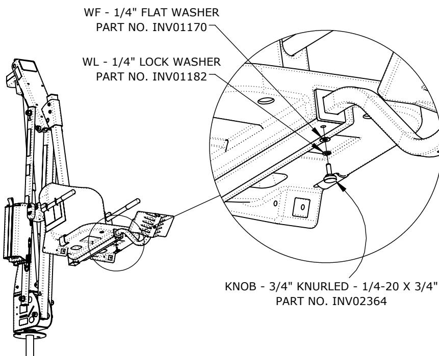
STEP 3) INSERT THE FOOTREST ASSEMBLY INTO THE 2"X2" SQUARE TUBING THAT SUPPORTS THE SEAT UNTIL THE PLASTIC INSERT OF THE FOOTREST ASSEMBLY SITS FLUSH AGAINST THE END OF THE 2"X2" TUBE. USING THE SUPPLIED 1/4" HARDWARE, FASTEN THE LEGREST ASSEMBLY TO THE 2"X2" TUBING.
