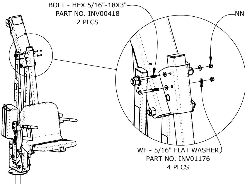
STEP 2) SLIDE THE SEAT CRADLE ASSEMBLY UP THROUGH THE TOP CASING OF THE MAST ASSEMBLY AND CONNECT USING THE SUPPLIED 5/16" HEX BOLTS, WASHERS AND NYLOCK NUTS. FOR STANDARD POOL CONFIGURATION THE SEAT CRADLE WILL BE CONNECTED AT THE TOP TWO HOLES. HOWEVER, THE SEAT CRADLE CAN BE ADJUSTED UP TO 6" HIGHER, IN 2" INCREMENTS, IF THERE IS A NEED FOR IT.
